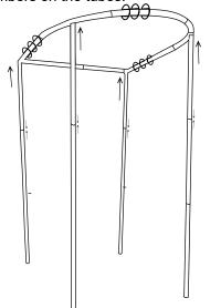
4. Connect the assembled frame with the base assembly as shown below.
