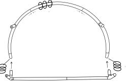
2. Snap and connect the tubes to assemble the bottom the same way.
