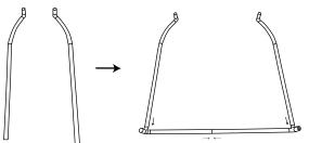
3. Snap and connect 4 supporting tubes with the top frame by matching the numbers on the tubes.
