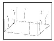
Set the assembled base on the ground so that the Short Bars are facing upward.
