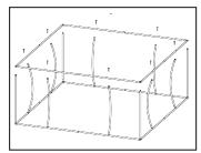
Attach the 2nd set of long bars (A) to the top of the curved short bars (E) using the remaining short screws (D).
