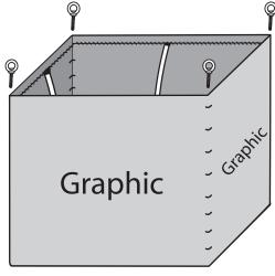
Align all holes then insert long screws and hand tighten
