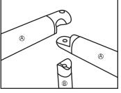
Align the ends of the each side as show, making sure to align the grooves in each piece to properly align.
