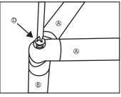
Using the Short Screws (D) attach the Short Bar (B) to each corner as pictured.
