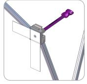
Attach the female arm by popping it into the hub. Fasten the screw through the steel plate hole and the velcro webbing tapping into the female arm.
