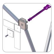
To dettach the female arm, remove the screw, steel plate and velcro webbing. Pull the arm off the hub.
