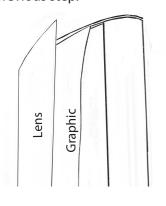
5) With graphic and lens in place slide hand from center to edge to make sure lens is secure.
