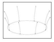
Set the assembled ring on the ground so the Short Bars (B) are facing upward. Position your unzipped graphic underneath the ring.
