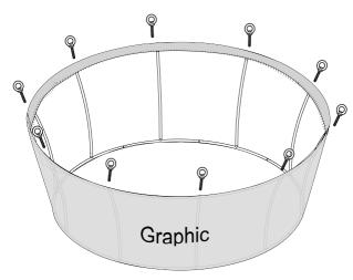
Align all holes then insert long screw and hand tighten.
