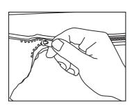
Once all long screws are in place, lift the inside of the graphic and zipper The sections together.
