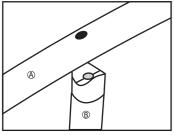
Choose one of the circular rings and align the Short Bars (B) with the holes in the middle of each section.
