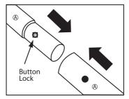
Connect (7) Long Bars (A) end to end to form a closed ring. Repeat this step to form another ring. These are the top and bottom supports for your graphic.
