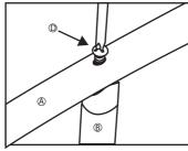
Attach ring to middle supports (B) using the short screws (D).
