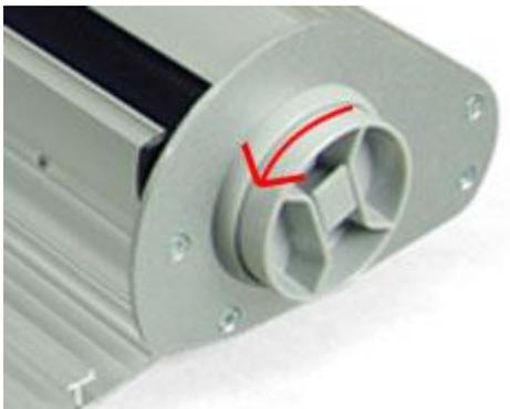
The rotating knob is used to add tension to the spring. It should only be used when replacing the banner. Applying too much tension to the spring will damage the unit. Tension on the spring will increase as the banner is raised.
