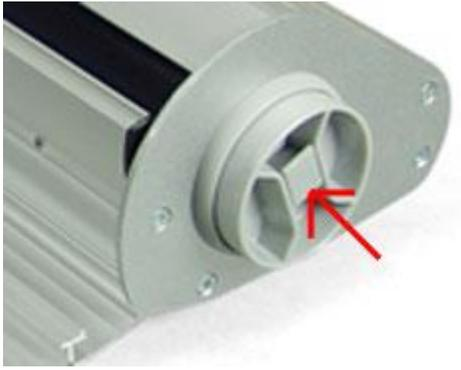
The tension release is used to release tension on the retraction spring. This is only required if the banner is to be replaced, or if there is a problem with the unit. **DO NOT** release tension on the spring while the banner is in the raised position, as damage to the spring may occur. Remove the banner once tension has been released.
