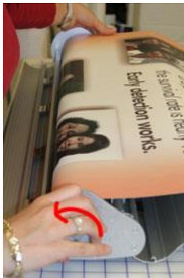
9. Begin adding tension by turning the knob counter-clockwise. After a few turns the system will start to pull the banner onto the rolling drum. Guide the banner to ensure that it is centered on the drum.
