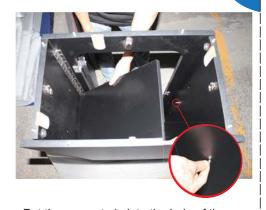
Put the support pin into the hole of the panel, put the fiex divider on it
