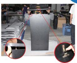
Put the top panel on the counter with lock catch, align the hole and screw
