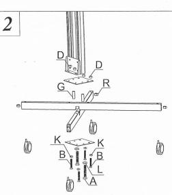
Fixed the pedestal to the inner screw thread tube with the bolt(B), washer(K)and screw nut (D) with the bolt(A),washer(L)
