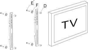
7. Adjust the height of the Hanging Panel as needed. Hang the TV with brackets attached onto the Hanging Panel, and insert the Safety Bar at the bottom of the Hanging Panel as
