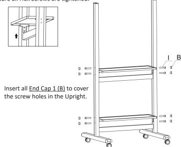
5. Mount the Hanging Panel onto the assembled Uprights by using the hardware provided. See image below. Insert (2) End Cap 2 (C) into the top of uprights.
