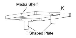
4. Place (1) assembled shelf in the middle of Left and Right Uprights 6. Mount (2) mounting brackets to the back of the TV and align corresponding holes on them. Fit (1) Rectangular Tube between (2) T Plates, then screw (2) Hex Screws (I) From each side. Assemble the other Shelf and Rectangular Tube the same way. Be sure all Hex Screws are tightened.
