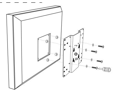
\*Please Note: If the mounting holes in the monitor are in a recessed area, spacers (provided) must be used to bring the plate to the proper installation depth. If the display mounting area is flush, the spacers are not required and plate is mounted directly to the monitor.
