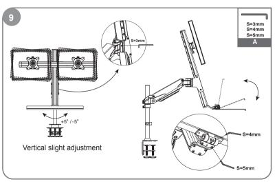
Use a hex wrench to adjust the two screws below the keyboard tray If you want to adjust the tension.
