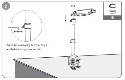
Lift the gas spring arm and put it on the locating ring and then insert the pole cover.
