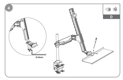
Connect the keyboard tray with the aluminum profile component.
