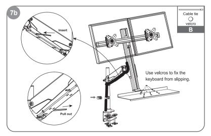
Use cable tie to manage large number of cables. Use cable clip to limit cables close to steel pipe.
