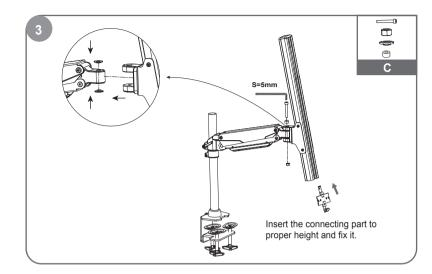
Connect the aluminum profile component with the gas spring arm.
