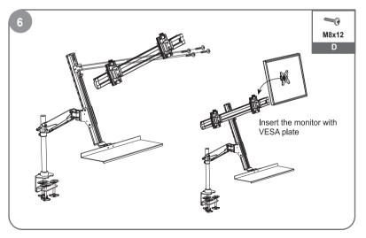
Attach the aluminum profile to the connecting part.
