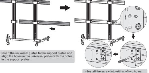
• Tighten all screws but do not over tighten!
