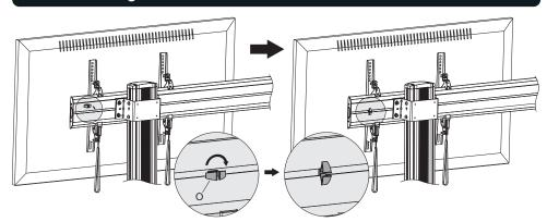
Insert the cable clamps horizontally into the plate slots, then turn the cable clamps to the vertical to secure them.
