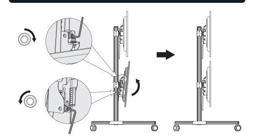
If the displays tilted down, rotate the adjustment screws as shown in figure.
