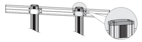
Attach the top covers to the columns using the appropriate screws. Tighten all screws with an Allen key.
