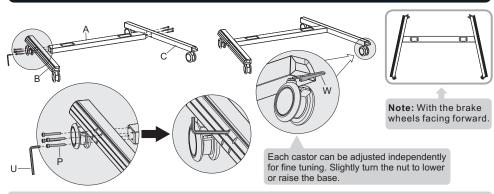
Attach the left and right base to the middle base using the appropriate screws. Tighten all screws with an Allen key.
