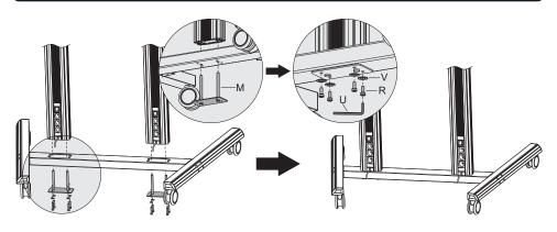
Attach the columns to the assembled base using the connecting pieces, secure them with the appropriate screws. **NOTE:** Lock the brakes on the casters to avoid any sudden movements during installation.
