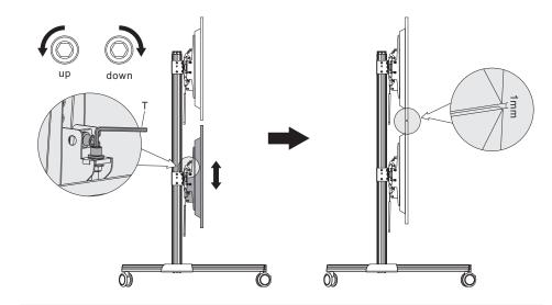
Rotate the adjustment screws as shown in figure to make a one millimeter gap left between the upper and lower displays.
