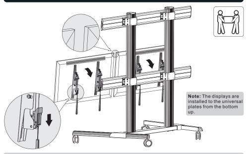
Lift the display carefully and pull downward two straps at the same time, then hook the adapter brackets to the universal plates. Fasten the adapter brackets to the universal plate by releasing the straps.
