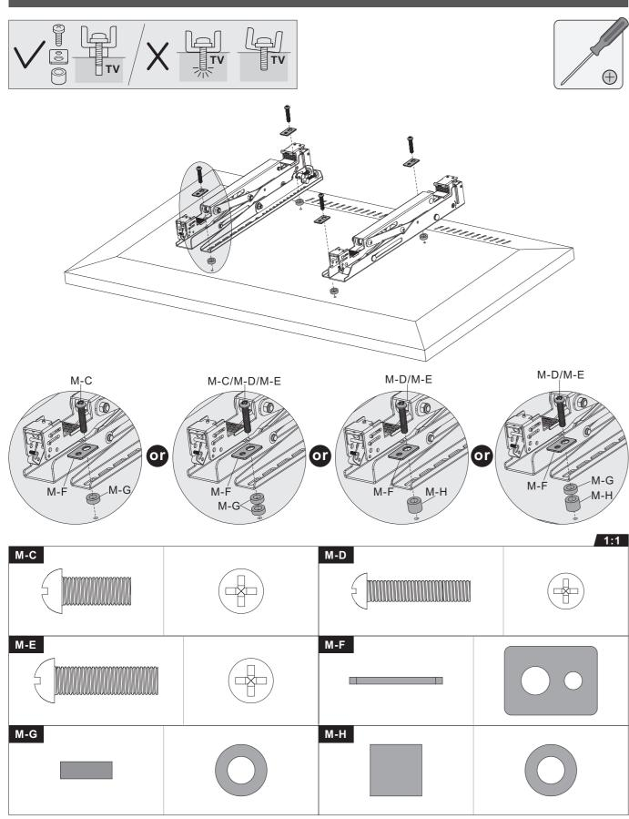
Note: Choose the appropriate screws, washers and spacers (if necessary) according to the type of screen.
