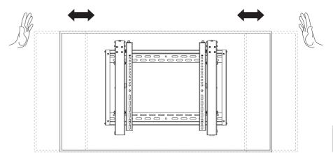
Push the display to left or right to enable fast alignment.
