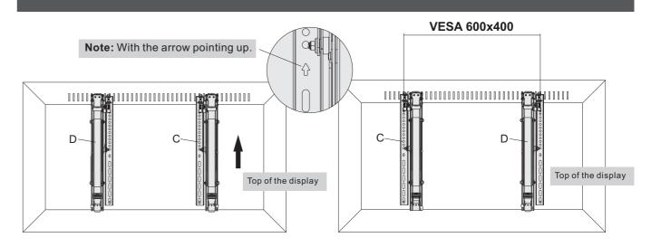
For VESA 600x400, the positions of "D" and "C" are exchanged.
