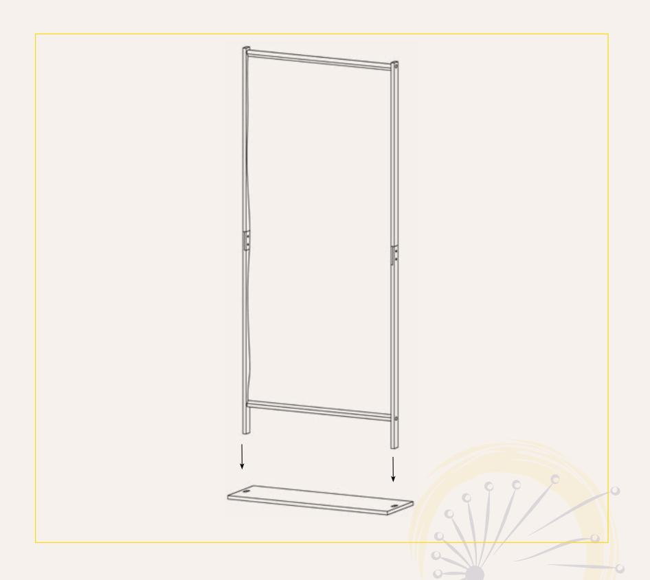
4. Insert both side poles into the Base (E). Test to make sure the whole unit is stable.
