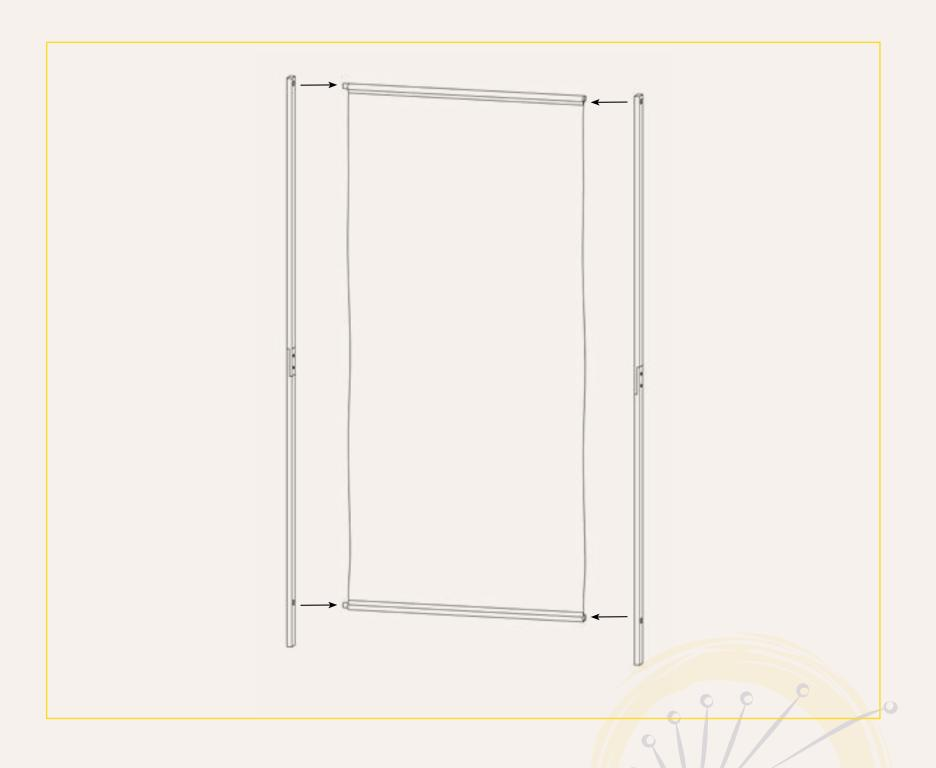
3. Insert the round bar into the pre-drilled holes on the side poles as shown.
