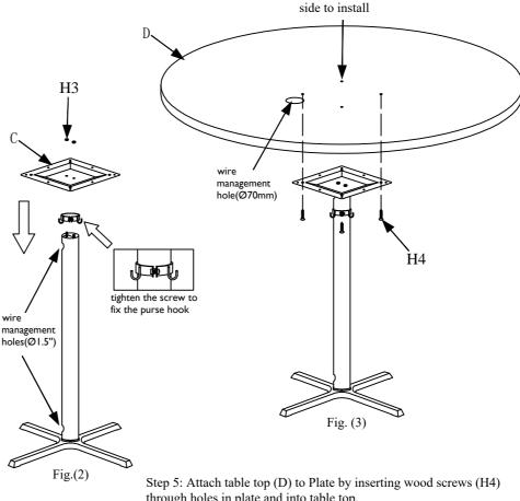
through holes in plate and into table top.
