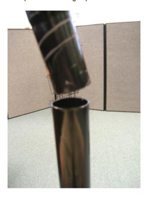
Step 4: Slide wire frame onto assembled poles.
