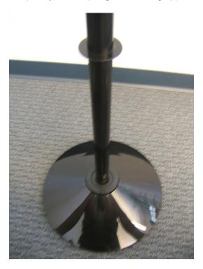
Step 2: Slide bearing onto pole until it is seated on the flange.
